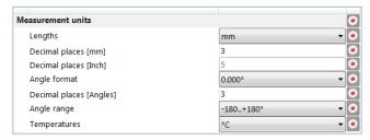
Now all parameters of the measurement units group and the report settings can be recorded in a measuring program. This allows the reports to be reproducibly generated with the selected settings.
