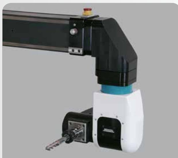
**Additional emergency stop on the milling head (Excalibur)**
