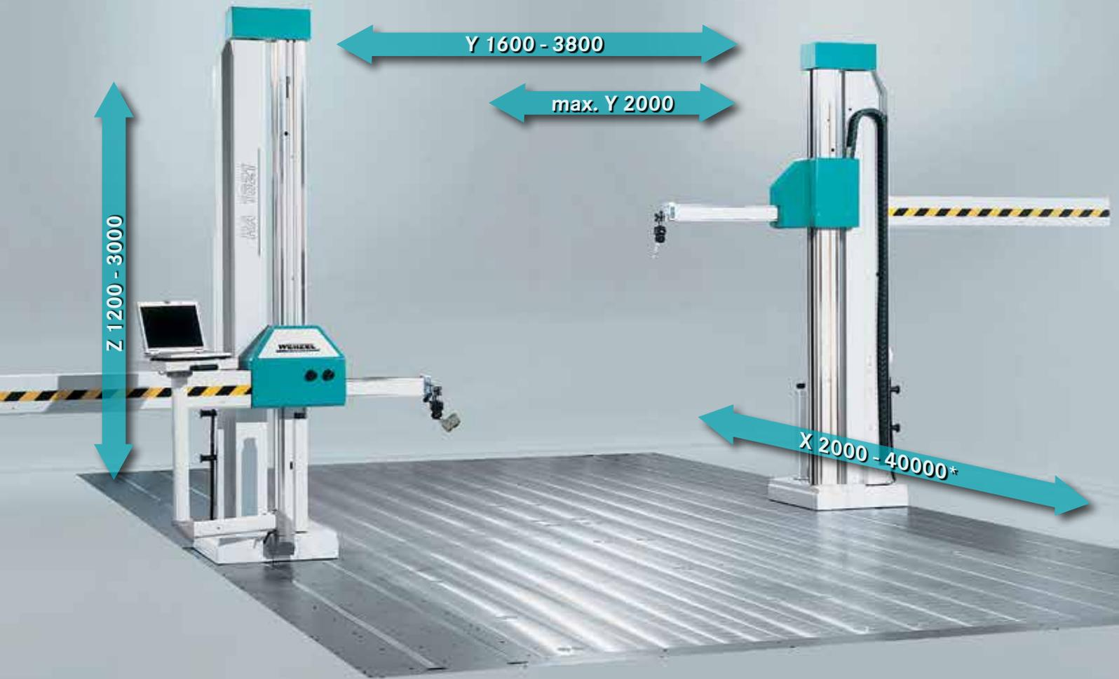
\* All machines are available as standard up to X = 40.000 mm, 500 mm increments, larger X- and variable Y- and Z-ranges on request.
