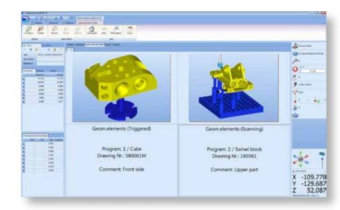
The Program Launch Panel allows Production Operators to execute CMM programs at a single click and prevents access to programming and edit tools.
