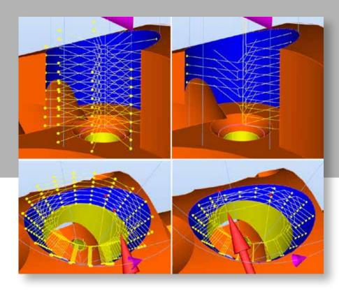
Where a geometrical element is not whole 'Consider Model' function drops measurement points only on existing surface of feature (Right hand images) rather than the complete theoretical surface (Left hand images).
