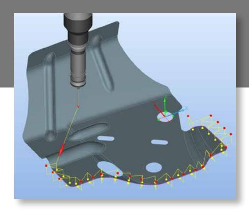
Trimming edge measurement with automatic point distribution on reference surface and edge.
