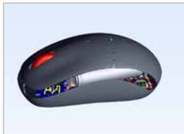
Side view into the partially opened housing. The position of the individual parts in relation to each other can be analyzed in the assembled state.
