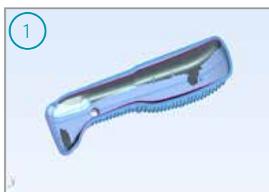
Alignment of actual- to nominal component
