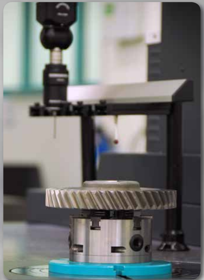
The high-precision rotary table enables the flexible and precise measurement of gears and rotationally symmetrical components.
