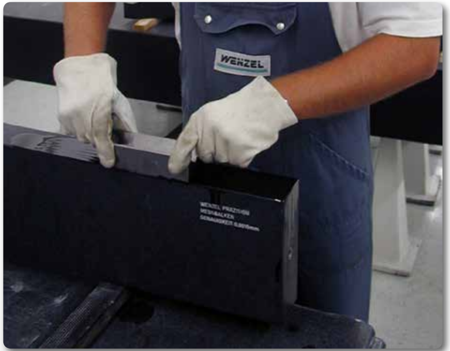
The granite is meticulously lapped by hand to ensure highest level of accuracy.
