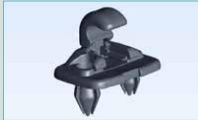
The CT scan generates a complete 3D surface model of the part. This includes internal and external geometries.
